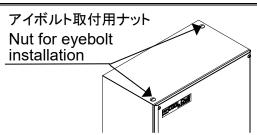
OCA-H800BCS has two nuts on top for installation of eyebolts. Please lift up evenly using eyebolts whenever lifting up a cooling unit. Lifting up one side only may result in breakdown or damage of the product.
